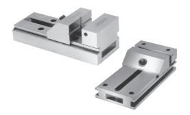
Angled channel provides extra jaw capacity. Jaw can be opened or closed without unbolting from work surface. Squareness and parallelism within .0002". V-237-S1 has recessed pockets at both ends for clamping. Vees machined in face of moveable jaw and 12 stepped channel which eliminates side holes are available on some models.
