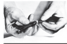
1. Slip screw into end of wrench.
