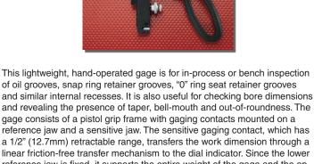
reference jaw is fixed, it supports the entire weight of the gage and the operator's hand, thus preventing incorrect gaging pressure and false readings. Furnished with jewel bearings, in case.
