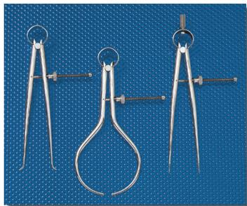
Designed for toolmakers and all good mechanics who require finer adjustment and better balance so a more sensitive feel can be obtained. The fulcrum stud is hardened and the bearing surfaces of the legs are large enough to prevent any side deflection. The bow spring is strong and flexible, and the adjustment is centrally located in the legs to assure smooth action.
